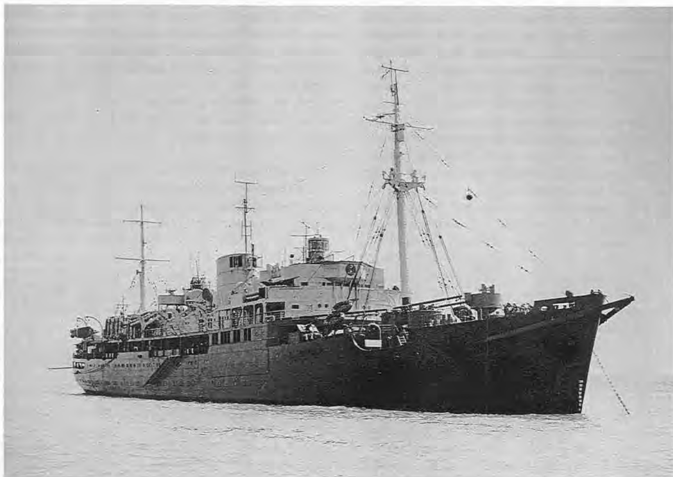
LSH, HMS BULOLO, operations HQ ship during the invasion of Sicily. Note the armour-plate belting along the hull at upper deck level, adjacent to the central receiving room, signal control and cypher offices. Immediately above these spaces, at bridge deck level, were the Navy and Army operations rooms, support control, signal distribution lobby, and the intelligence office - all externally armoured. Above these, at boat deck level, were the war command and the wireless transmission rooms. Note also the projection from the bow. Does a reader know whether this was used in the detonation of acoustic mines, or for paravane sweeping? ((Imperial War Museum. Neg. A23597)
