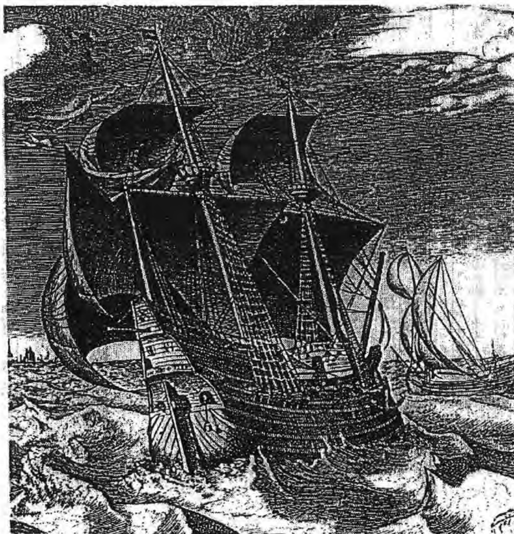
An engraving by Frans Huys after Pieter Bruegel, 1565, of a forerunner of the Dutch fluit. The fluit or fluyt was a cargo carrier which had a longer length to beam ratio than the usual vessel of the time. They therefore were good sailers while retaining the ability to carry a good deal of cargo on a reasonably shallow draft.
