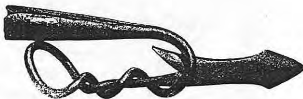
Bent double and twisted like taffy by the gyrations of a wounded whale, this harpoon was fashioned from malleable iron, which would bend rather than break under stress. Harpoons were often mangled during the hunt, and though this one must have seemed beyond repair, most were recovered and straightened.
