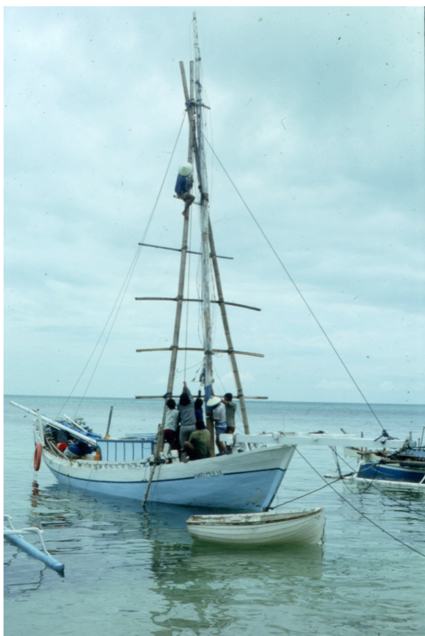
Lifting out the old mast
