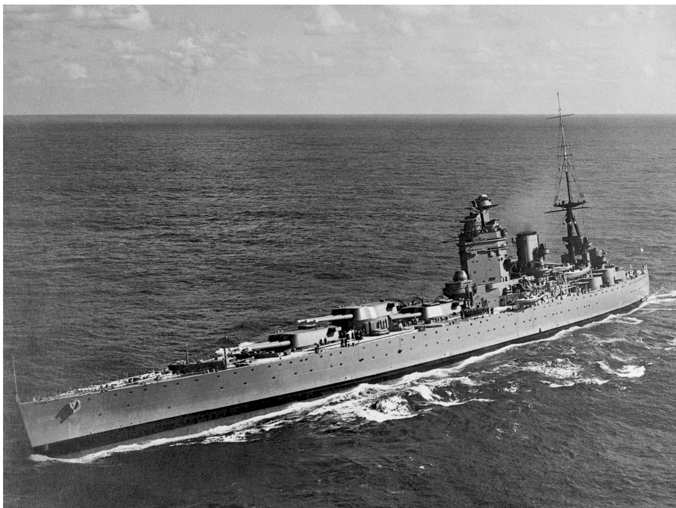
A photograph of HMS Rodney which carried 9 16-inch guns in 3 turrets, plus 12 6-inch guns. Launched in 1927 the 33,900 ton battleship had 14-inch side armour, and a speed of 23 knots. Rodney took part in the sinking of the Bismark.
