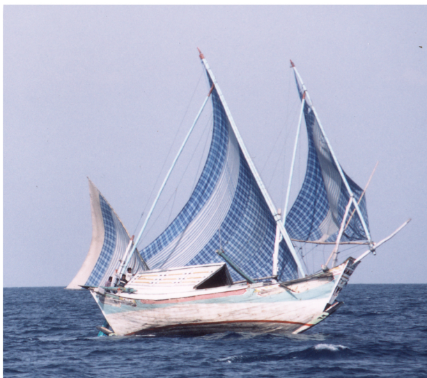
A janggolan flying light with no ballast and hard on the wind
