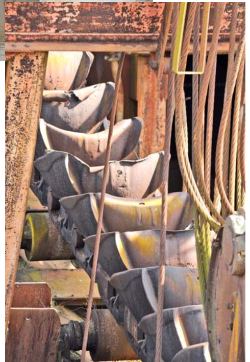
A few of the 110 buckets, each of which weighs 1.6 tons and holds 12 cubic feet
