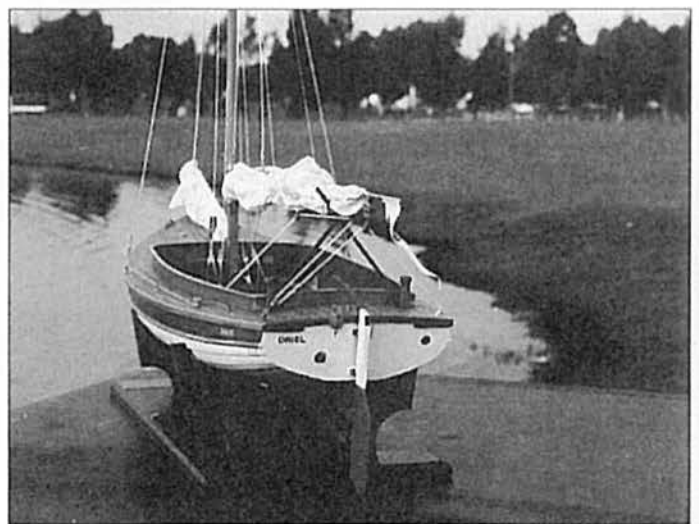
After end of the model, showing the shape of the transom, with exhaust and bilge pump outlets. Photographs by the author.
