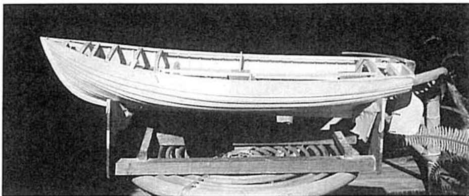
The basic hull finished, with rudder temporarily in place.
