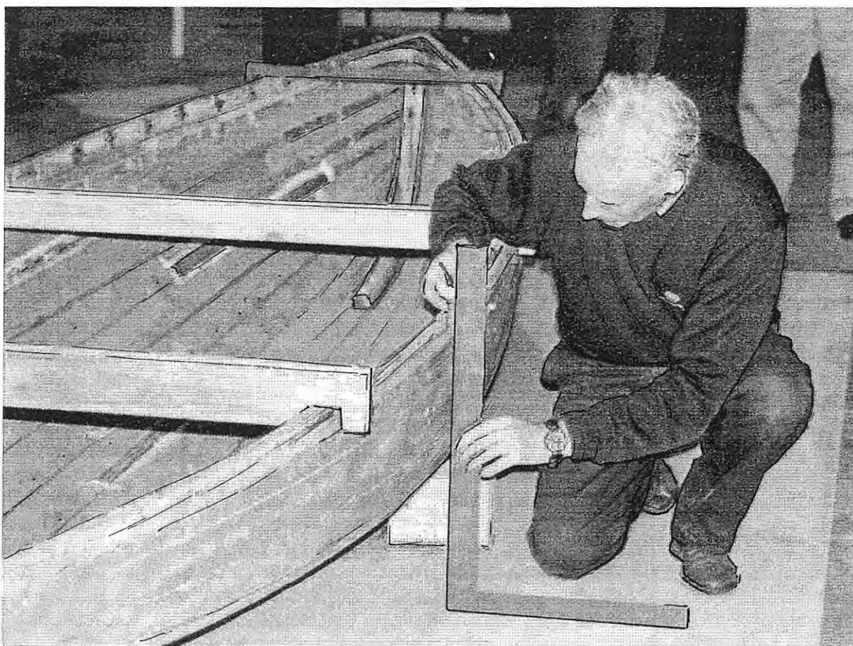
Bill Leonard demonstrating how to take the lines off a dinghy using the method described in this article.
