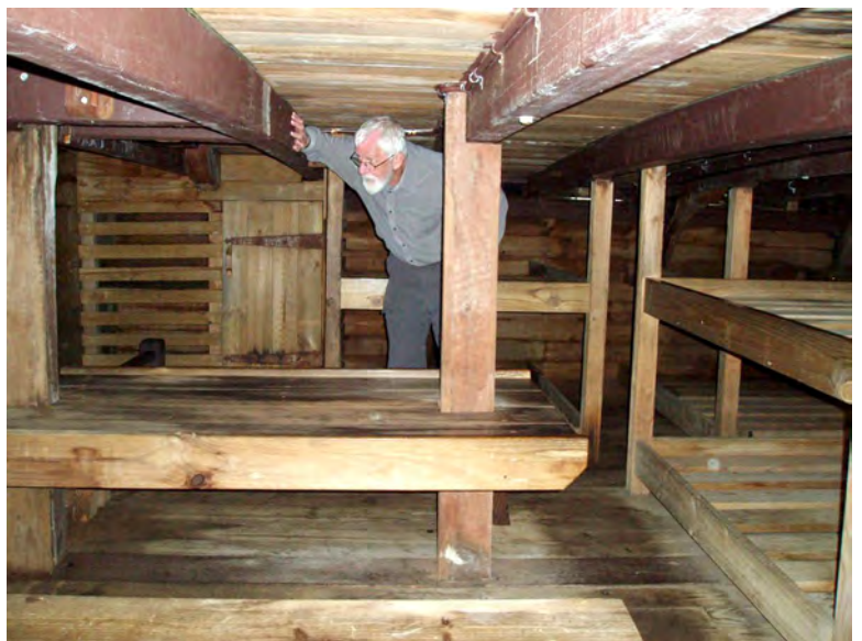
Amity's 'tween deck with copious 4ft 11in headroom between beams. Mess table in foreground, two-upon-two berths (right) and a brig=upon-brig (left) - records show Amity carried a 'detention cell' for prisoners of bad character.
