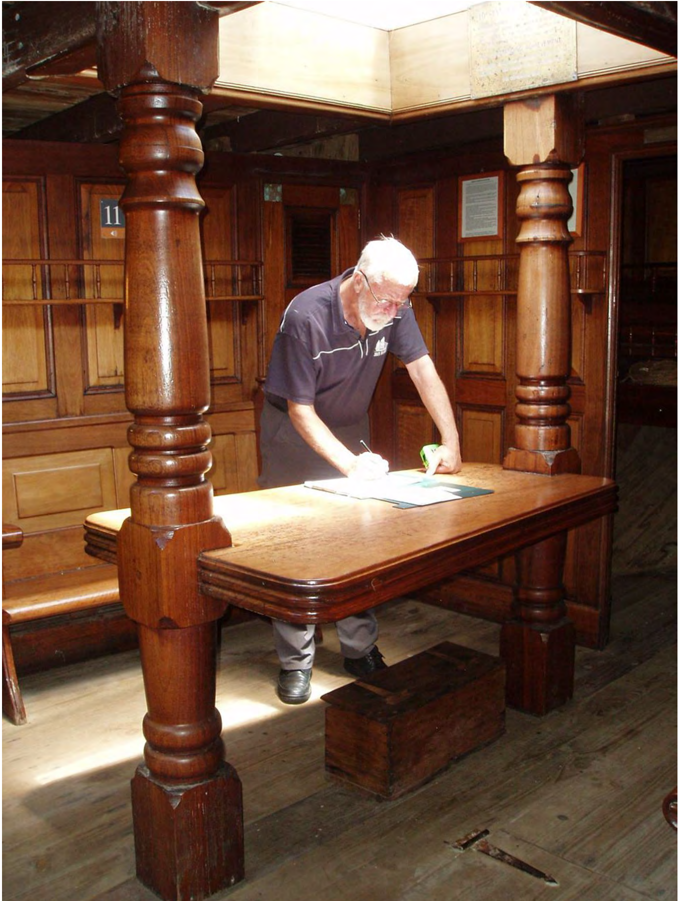
Measuring up the after cabin for the Inboard Longitudinal Section drawing. The teak and mahogany panelling came from old railway carriage doors supplied by the Railway Workshop, Bassendean.
