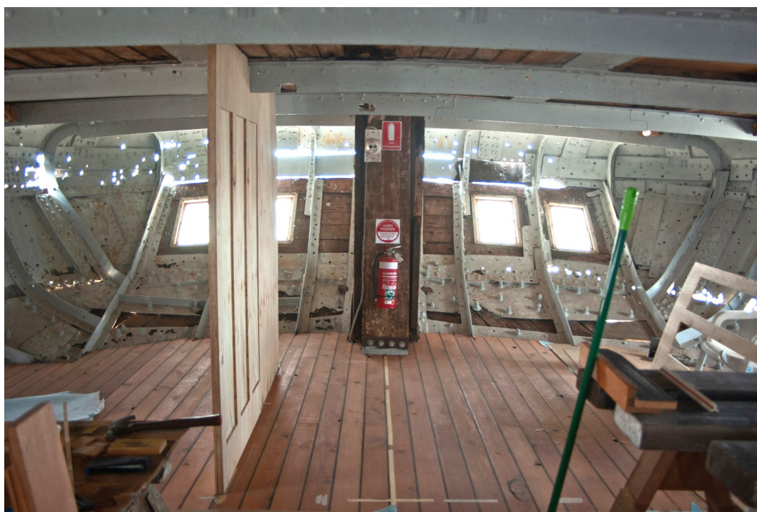
First Class New decking,, and replica first-class cabins under con- struction. Plenty of daylight showing through holes in the hull
