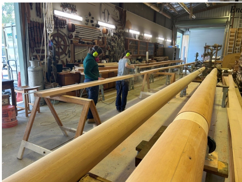
Robin Hicks's Sailmakers & Riggers Shed – masts and spars for STS Leeuwin II
