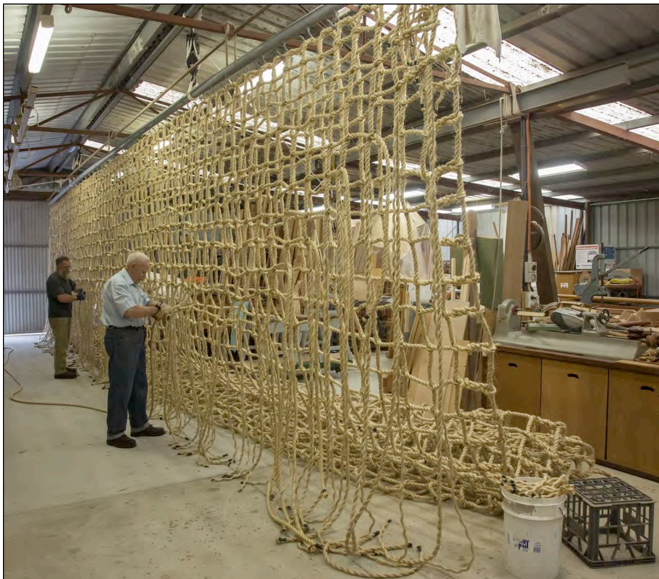
Robin and Barry Hicks at work on another 'possum net' – otherwise known as a helideck net. Laid out flat on the helideck of a ship and hauled tight, it is used under certain weather conditions as an aid to landing, particularly if the vessel is rolling and moving about.
