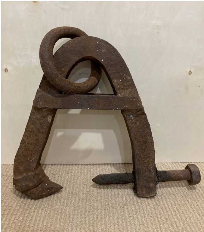
Stan Austin's father, Lionel Rosser Austin; blacksmith, carpenter, fisherman and boatbuilder, made this massive clamp to lift the 31cwt (1.57 tonne) lead keel from the wreck of the Lenita.
