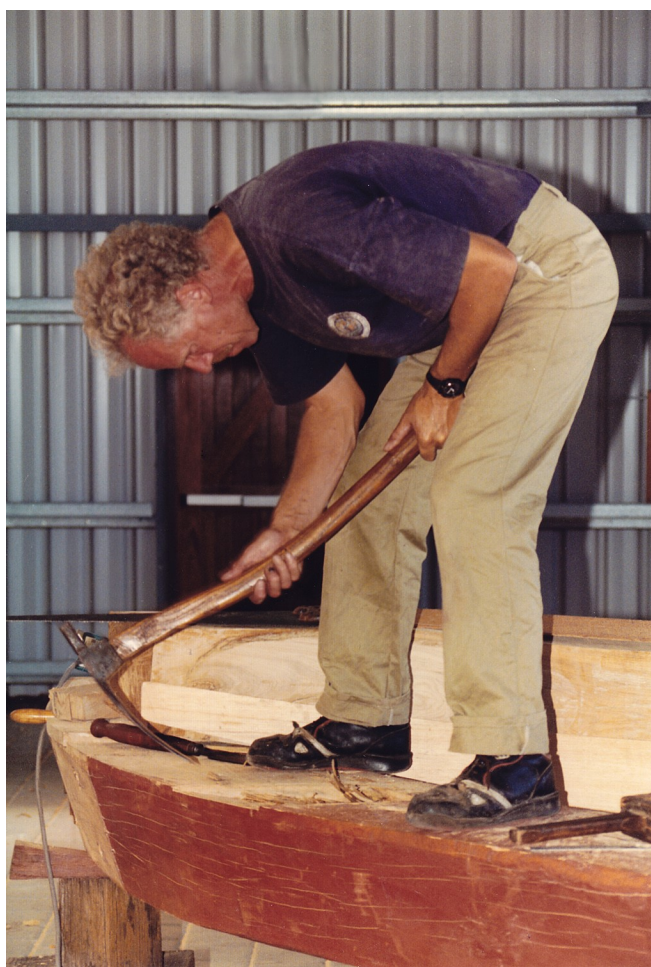
Bill Leonard, at work on part of the stern of the Duyfken . He was a superb adzeman – this being a very tricky tool to use.
