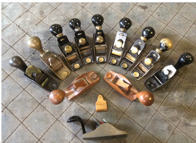
Robin's collection of Stanley No.100 squirrel tail block planes. The two wooden patterns for casting Miller squirrel tails are in the centre.
